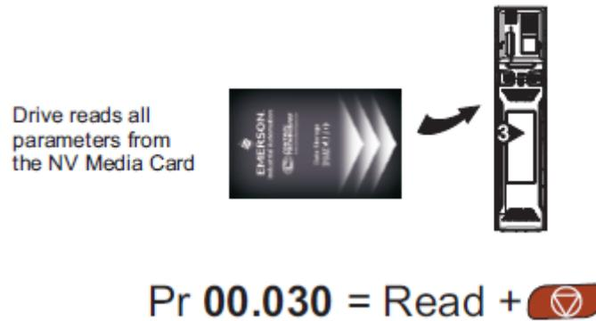
A small flashing period will flash next to left hand side of '00.030' during the programming of the M700 drive. Parameter 00.030 will change back to 'None' once the programming is complete. Cycle power to the drive and the newly programmed M700 drive is now ready for use.
