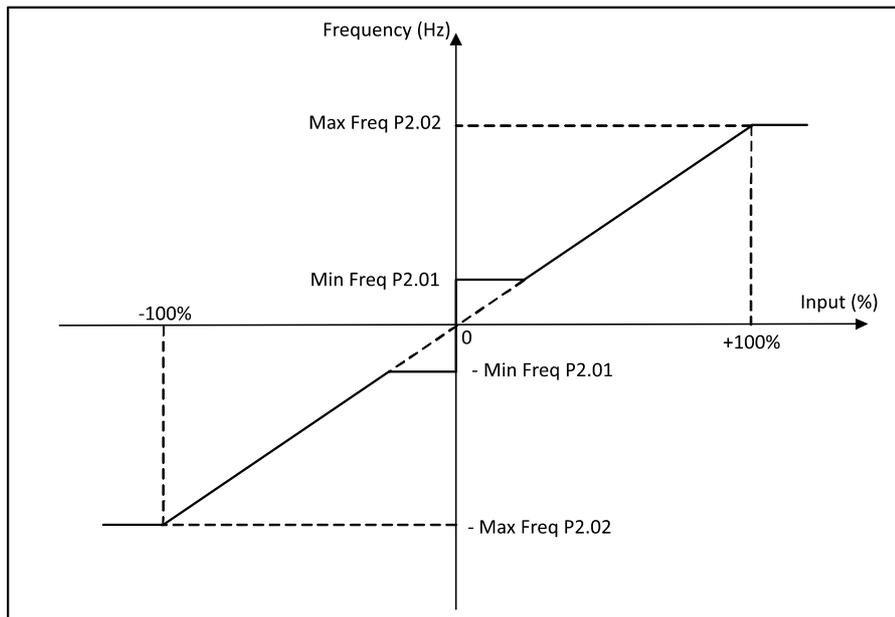
**NOTE** If this parameter is set to 0 (None), the drive will run at the *Minimum Frequency Limit (P2.01)*.
