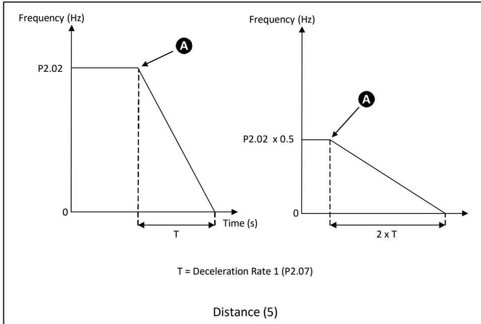
**A** is the point that the 'Run' signal is removed.
