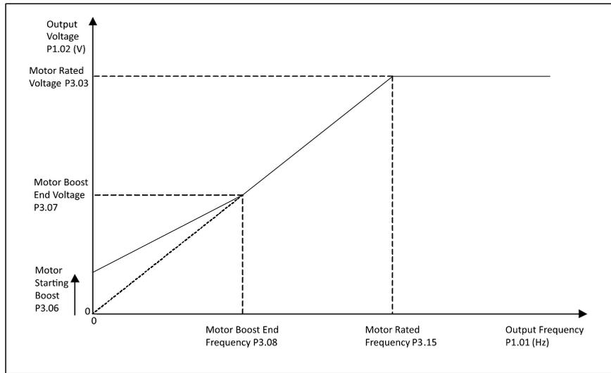
For Linear V to F, the voltage to frequency characteristic can be adjusted at two points, 0 Hz where the starting boost voltage is set in *Motor Starting Boost* (P3.06), and *Motor Starting Boost End Frequency* (P3.08), *Motor Starting Boost End Voltage* (P3.07) which is the frequency and voltage point at which the boost level is tapered to.
