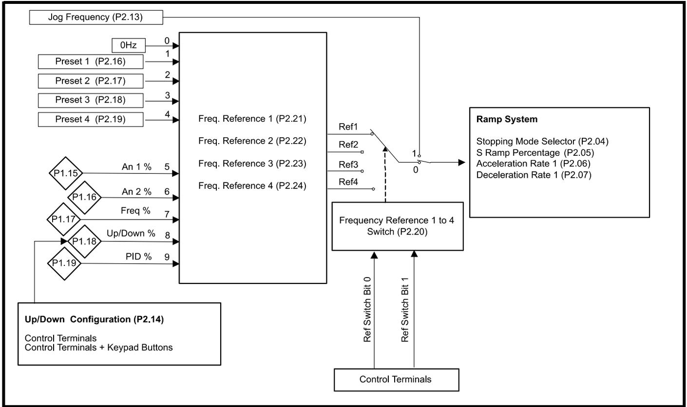
Reference Switch Bit 0 and Reference Switch Bit 1 can be selected as functions of the drive control terminals and use a binary system to switch between references as Table 7-1 describes.
