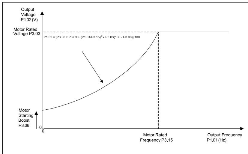
For Square V to F, only the starting boost is adjustable and the voltage output follows a square law from this point until the voltage reaches *Motor Rated Voltage* (P3.03) at *Motor Rated Frequency* (P3.15). At frequencies above this the motor voltage is constant.
