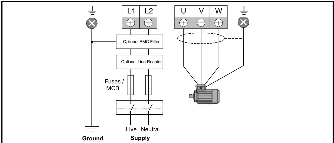
For dual-rated drives (S100-xxDxx), single phase connections should be made to L1 and L2.
