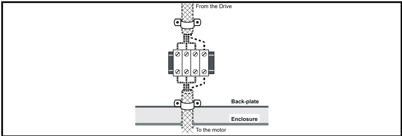
**Using a motor isolator / disconnect-switch**
