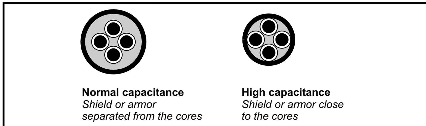
The maximum motor cable lengths specified in section 4.3.1 *Cable lengths*. are for cables that are shielded and contain four cores. Typical capacitance for this type of cable is 130 pF/m (i.e. from one core to all others and the shield connected together).
