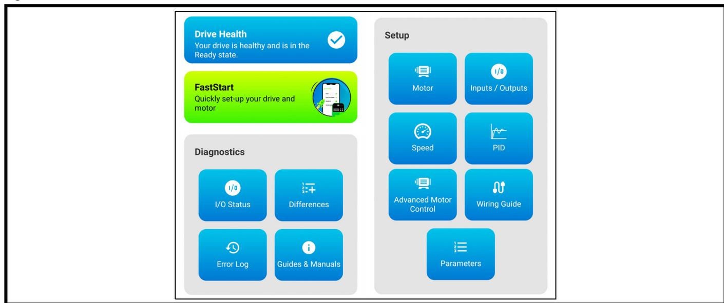
FastStart is the primary setup wizard, but more advanced commissioning can be done through the individual tools such as *PID* or *Advanced Motor Control*.
