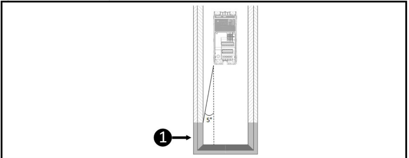
Openings for cables etc. must be sealed with materials meeting the 5VB requirement, or else have a baffle above. See Figure 3-2 for acceptable baffle construction. The distance below the drive where this applies to the enclosure wall = Distance from the cabinet wall to the drive ÷ 0.0875.
