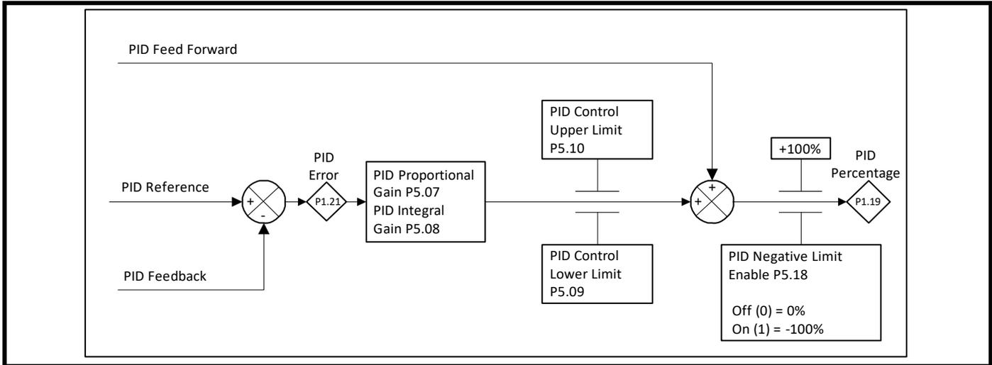
The response and accuracy of the process is dependent on the PID gain settings. See the descriptions of *PID Proportional Gain (P5.07)* and *PID Integral Gain (P5.08)* for setting instructions and more information. In the Commander S100 PID Controller the differential term is fixed to 0.
