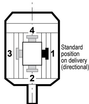
Position 2 not recommended (impossible on standard flange mounted (FF) motor)
