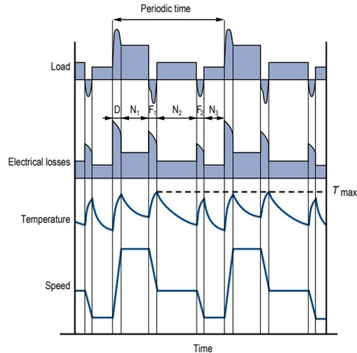
$F_1 F_2$  = electric braking
