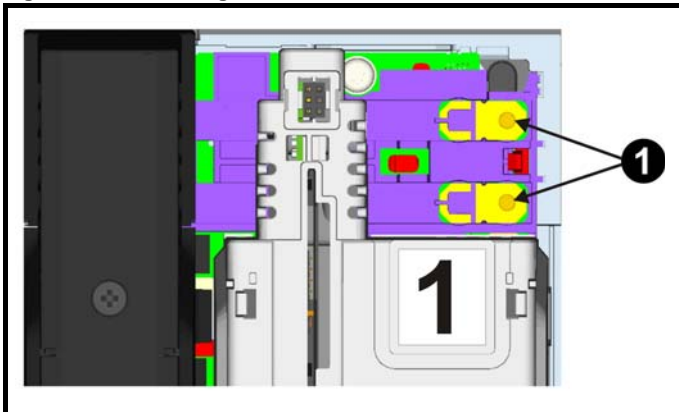
Figure 1-3 Removing the M4 screws from the DC busbars
